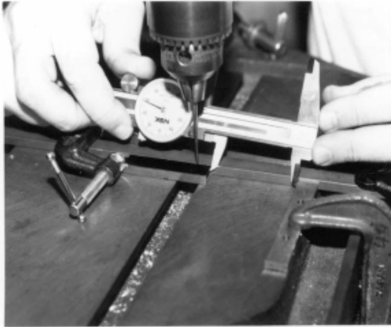
Figure 4: Drill press set up for accurately drilling waveguide filters. The dark object in the center is the filter to be drilled. The reference block is in the foreground to the right.
